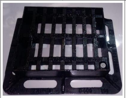
Rectangular Inspection Grating and Frame in spheroidal cast iron EN-GJS-500-7 with load bearing capacity over 250 kN (25tons), conforming to the load class C250 as set out by norm EN 124-2 2015
