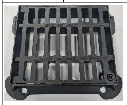
Inspection manhole cover in Spheroidal cast iron with load bearing capacity over 400 kN + 10% (40 tons), conforming to the load class D400 as set out by norm EN 124-2 2015
