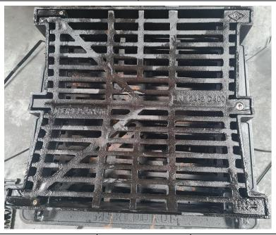
Inspection manhole cover in Spheroidal cast iron EN- GJS-500-7 conforming to norm UNI EN 1563:2004 with load bearing capacity over 400 kN (40 tons),conforming to the load class D400 as set out by norm EN 124-2 2015.
