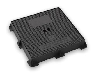
Inspection manhole cover in Spheroidal cast iron EN- GJS-500-7 conforming to norm UNI EN 1563:2004 with load bearing capacity over 400 kN (40 tons), conforming to the load class D400 as set out by norm EN 124:94.
