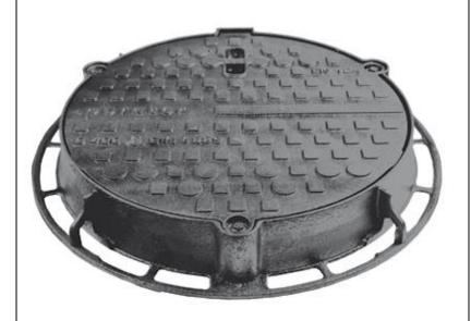
Inspection manhole cover in Spheroidal cast iron EN- GJS-500-7 conforming to norm UNI EN 1563:2004 with load bearing capacity over 400 kN (40 tons), conforming to the load class D400 as set out by norm EN 124:94.
