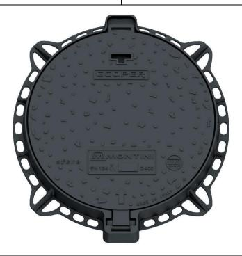
Inspection manhole cover in Spheroidal cast iron EN- GJS-500-7 conforming to norm UNI EN 1563:2004 with load bearing capacity over 400 kN (40 tons), conforming to the load class D400 as set out by norm EN 124:94.
