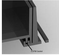
CROSS Section showing the watertight Seal Group 4
